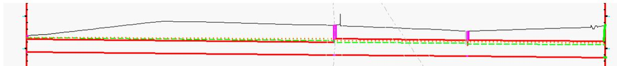
If the HGL is steeper than pipe slope (meaning surcharged) there is a good chance that the maximum size for the pipe type has been reached. For this lab this means that the structure file is incorrect. The structure file in the training directory should be adequate. The file can be checked via Drainage Options>General. Pipe sizes can be checked via Drainage>Structures File.
