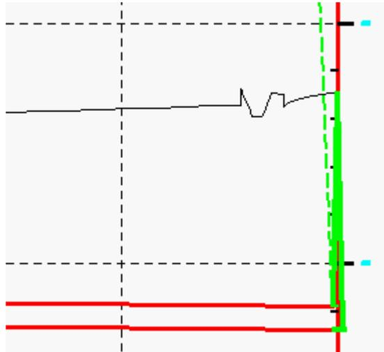
What is happening here is the network is terribly undersized for the flow coursing through it. The Condition field for all the structures is “Fixed.” S&S is not allowed to upsize the pipes to meet the design constraints.
